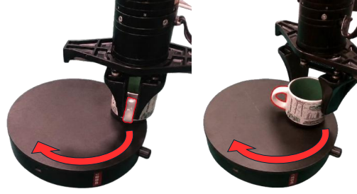
Figure 6: Fast-WAM (right) failure: the gripper reaches the cup but misses the rotating handle.
