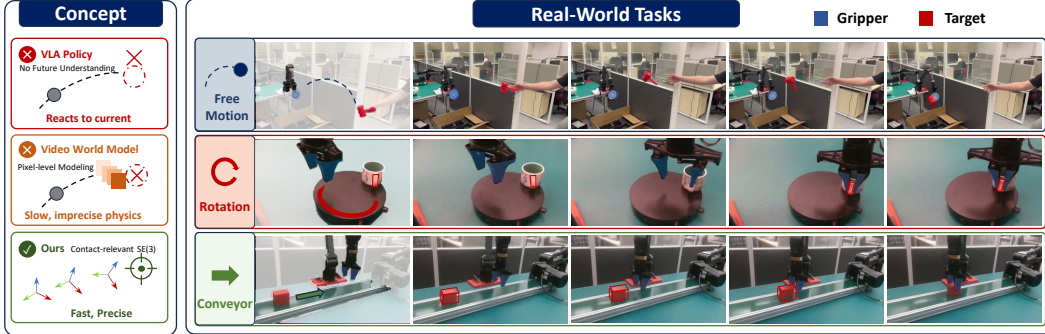
Figure 1: Left: Reactive policies act on the current object pose and fail under fast dynamics. Video world models predict pixel-level futures that are slow and physically imprecise. Our method predicts contact-relevant SE(3) state — compact, fast, and action-guided. Right: Real-world dynamic grasping tasks including parabolic catching, conveyor interception, and turntable grasping.
